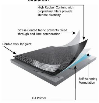
Strataflex® substantially reduces reflective cracking and delamination between the substrate and floor surface. Full floor coverage with Strataflex® will provide crack isolation protection for up to 10mm per lineal meter lateral substrate movement. The peel-and-stick membrane must be applied with C-I Solvent Based Primer and as soon as it is positioned, flooring can be installed immediately, minimizing down time and labour cost.
